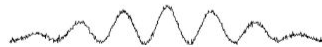
Fig. 7. The sum of 240 half-second exposures (120s accumulation time). The graph and image grayscale is 0-500 counts.
