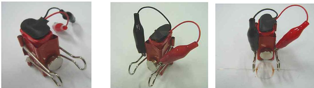
※ You can make 'battery snap with wire clamps' by yourself with a 9V-snap and two wire clamps. If you have none of these, you can replace it with two enamel strings(about 10cm long). Remove the enamel from the two ends of the string and attach them to +, - side of the battery. Then, connect them to each handle.
