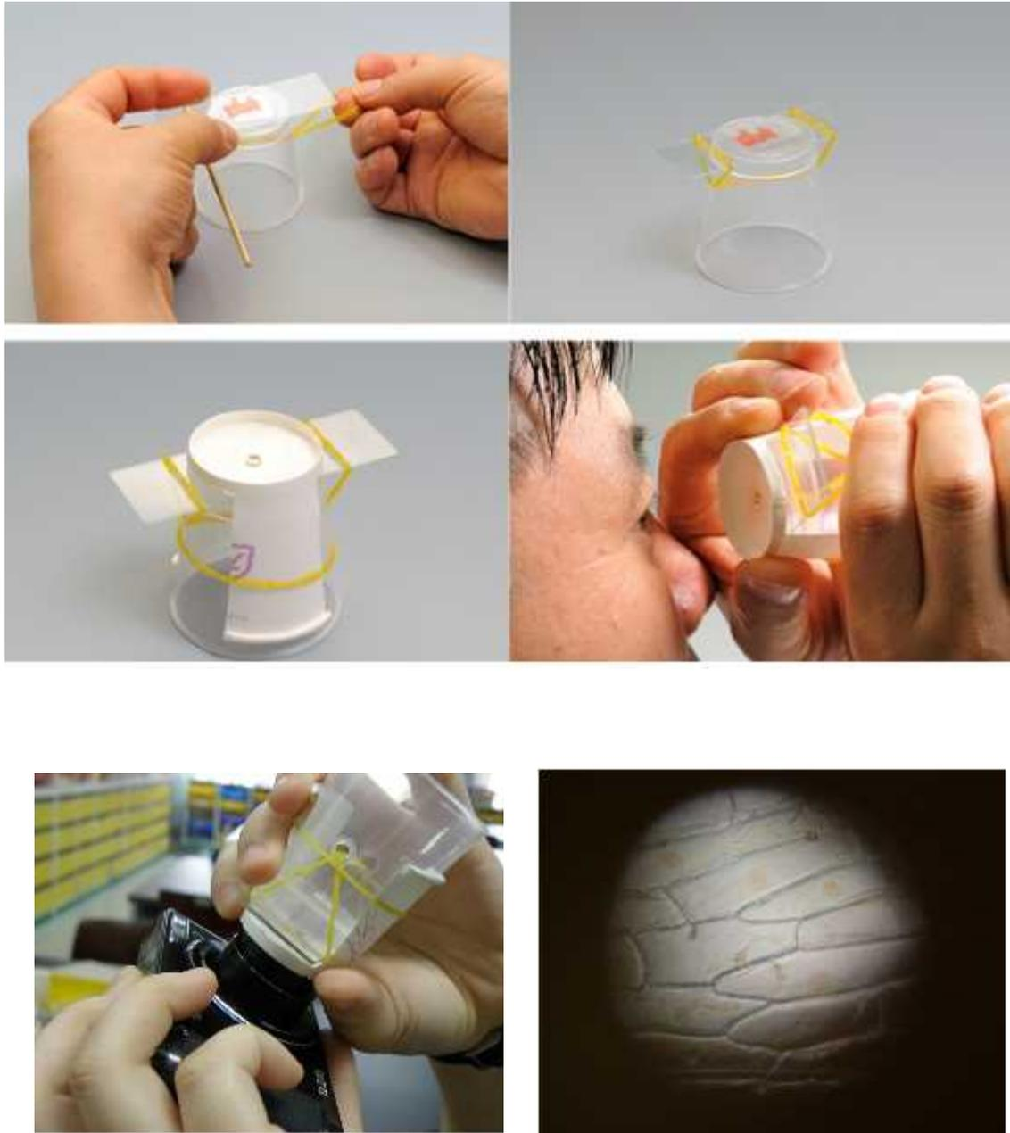
③ It is possible to observe when it is did below. OHP microscope can be separated and be replaced by a paper microscope. This is the same as using the rotary valve to move the object lens for magnification in a common microscope. Changing different holes gets the same results.
